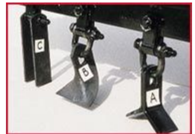
A: General Purpose Blade B: Lawn Blade C: Optional Scarifying Blade
